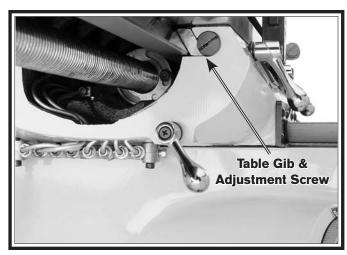
Figure 58. Table gib and adjustment screw underneath the left side of the table.
